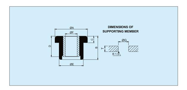
POLYBOND DUAL COMPRESSION (DC) mounts can withstand high static and shock loading to help isolate vibration, control shock, and reduce noise. These mounts are to be used with the right supporting member and snubbing washers.
