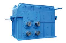
Special helical for pinion stand gearboxes designed and manufactured to suit the customer's specifications. Case / through hardened and profile ground steel gears with inclined tooth to transmit the torque between parallel shafts with minimum noise.
