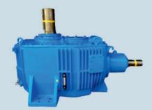
Case hardened and lapped steel spiral bevel gears to transmit the torque between right angle shaft. Unicase design with pumpless lubrication and three-point foundation.
